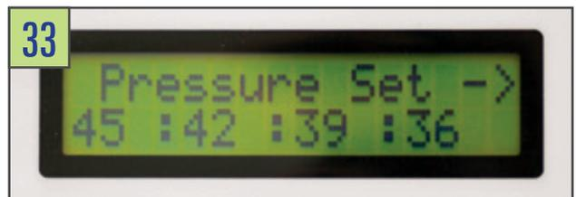
**34** You can increase the pressure by turning the SHUTTLE KNOB to the right, and decrease the pressure by turning to the left (pressure can range from 25 – 120 mmHg, increments of 1 mmHg).
