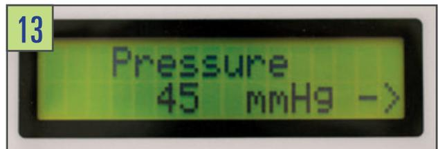
**14** You can increase the pressure by turning the SHUTTLE KNOB to the right, and decrease the pressure by turning to the left. (pressure can range from 25 – 120 mmHg, increments of 1 mmHg)
