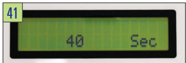
**42** Push the SHUTTLE KNOB to confirm the new cycle time.
