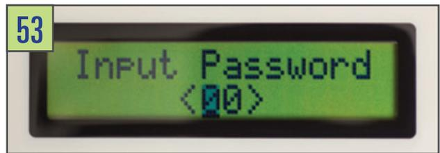
**54** Turn the SHUTTLE KNOB to select the first character of the password, press down and select the second character. Press down the SHUTTLE KNOB a second time to input the password. If the password is correct, the device will unlock and return to the menu screen
