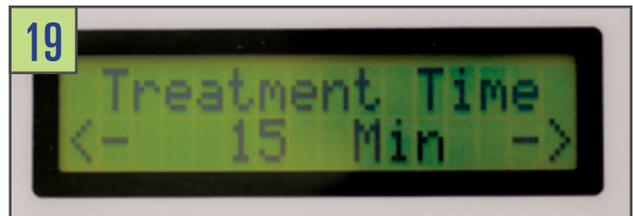
**20** You can increase the treatment time by turning the SHUTTLE KNOB to the right, and decrease time by turning to the left (treatment time can range from 15 – 180 minutes, increments of 15 minutes).
