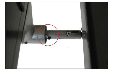
14. Make sure the slot on the spring loaded shaft engages the roll pin on the gear box.
