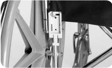
Fig. 15 - Chair bracket mounted on lower rear of wheelchair.
